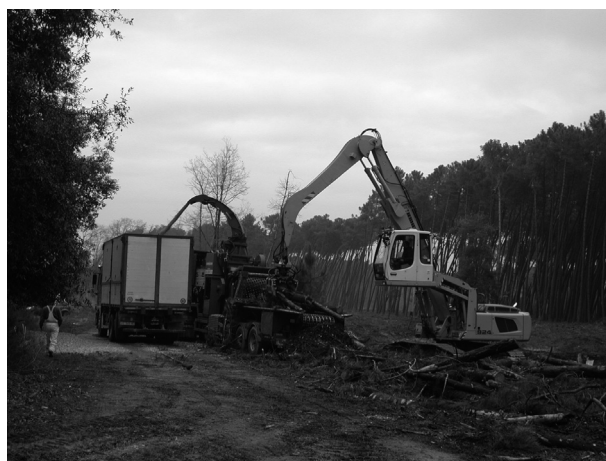
Fig. 2 Roadside chipping operation: the heavy chipper filling a chip van Slika 2. Iveranje na stovarištu: teški iverač puni kamion iverom
