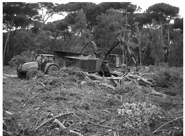
Fig. 1 Terrain chipping operation: forwarder-mounted chipper and chip shuttle
