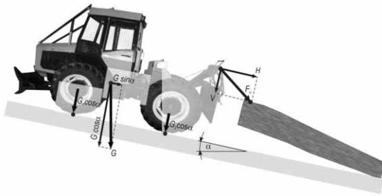
**Fig. 1** Distribution of forces during uphill timber skidding
