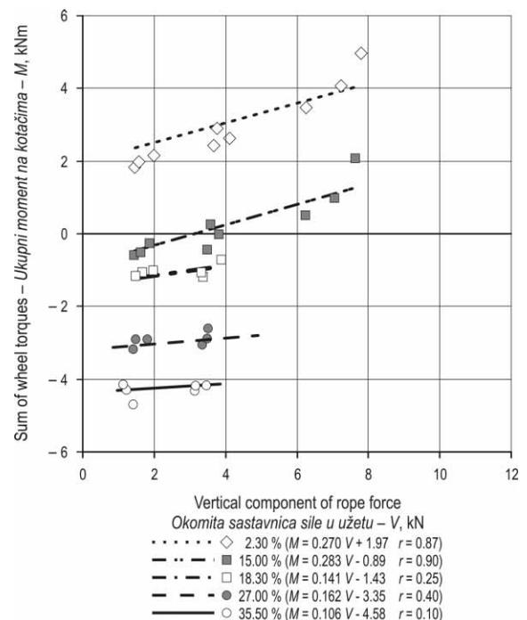
Fig. 9 Dependence of wheel torque on vertical component of rope force and downhill slope
