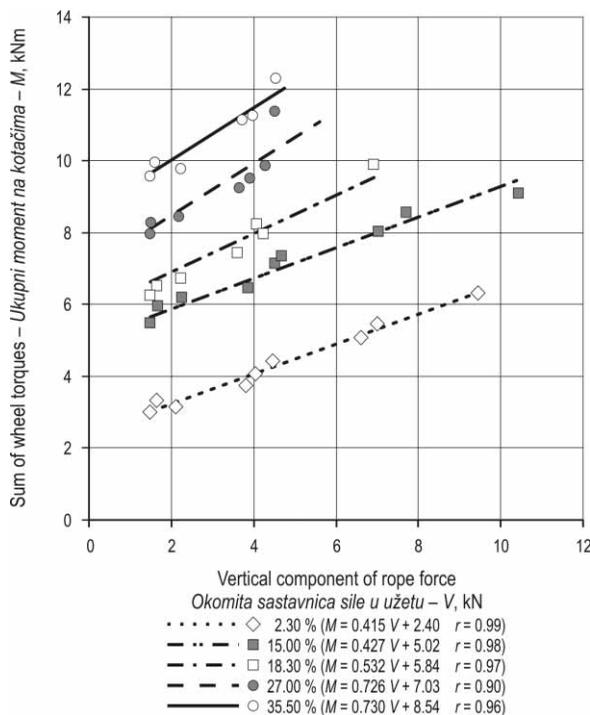
Fig. 8 Dependence of wheel torque on vertical component of rope force and uphill slope
