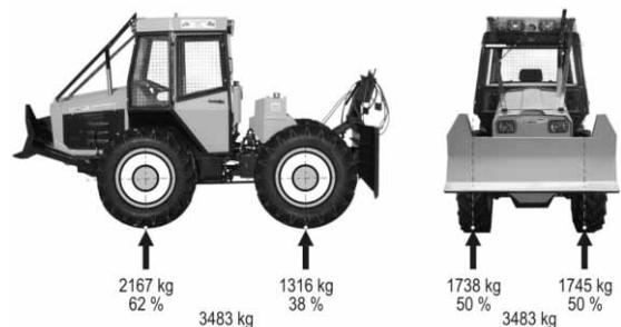
**Fig. 3** Mass distribution of skidder Ecotrac 55 V
