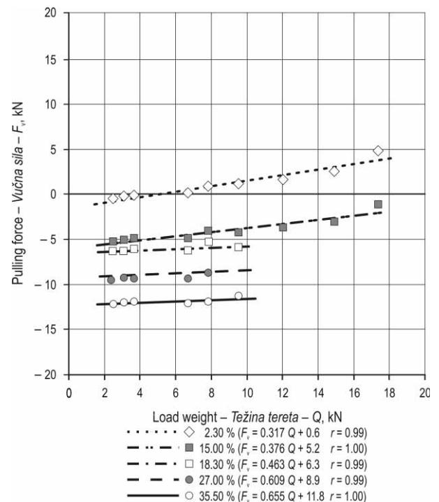
Fig. 7 Dependence of tractive force on load weight in downhill skidding
