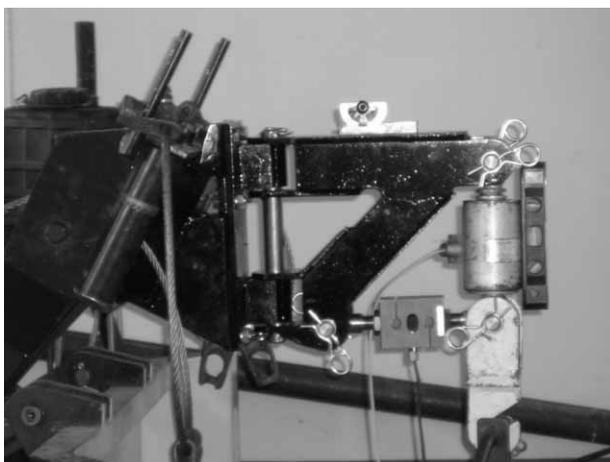
**Fig. 4** Carrier with traction and tension transducers
