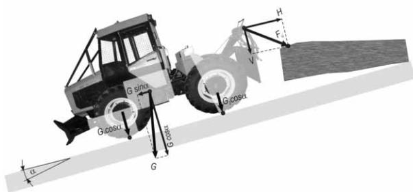
**Fig. 2** Distribution of forces during downhill timber skidding
