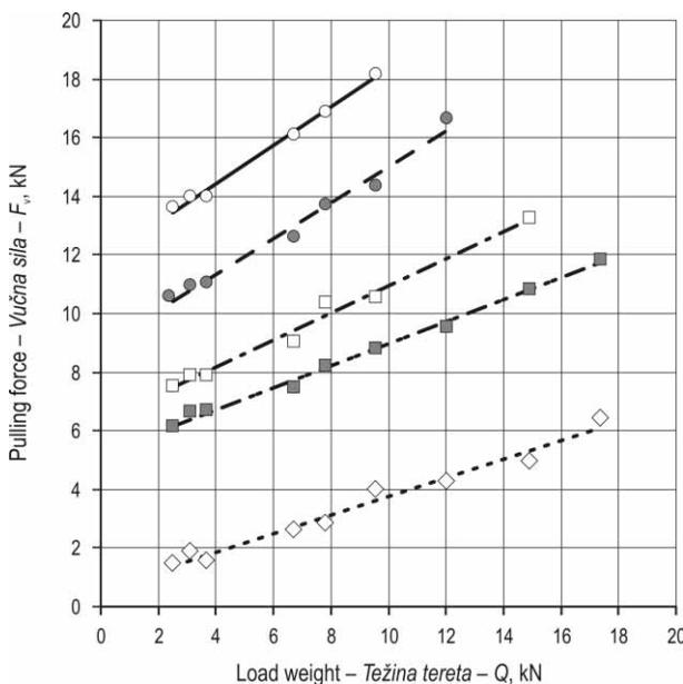
Fig. 6 Dependence of tractive force on load weight in uphill skidding
