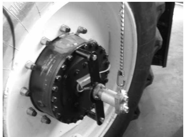
**Fig. 5** Preparation of final (planetary) drive
