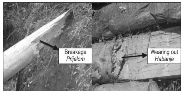
Fig. 2 Types of damage of transported logs
