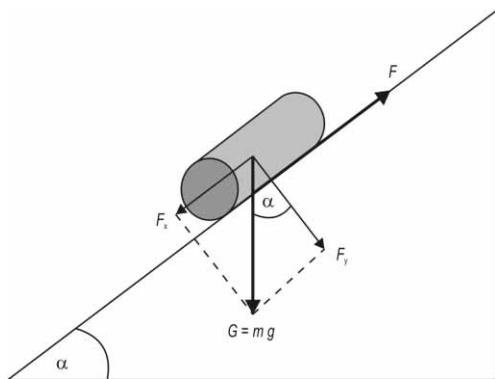
Fig. 3 The forces affecting the log skidded on inclined ground
