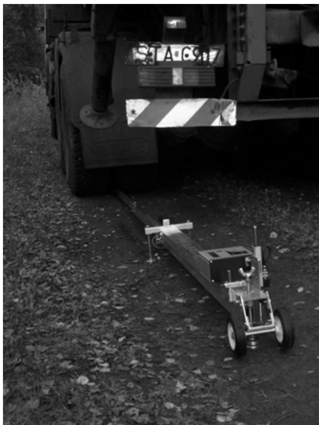
Figure 2 Measurement of the pavement deflection using Benkelman's deflectometer
