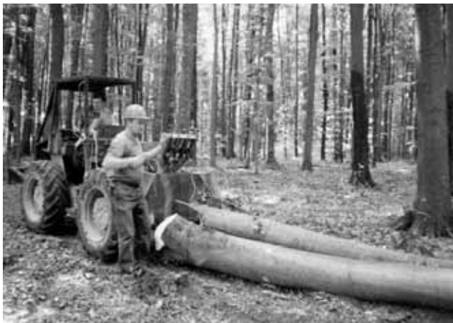
Figure 1 Cutter and tractor driver's work related to load hooking Slika 1. Sječač i traktorista pri vezanju tovara
