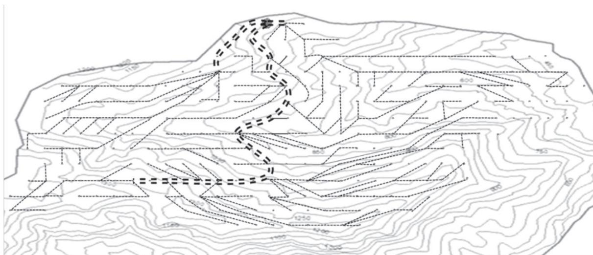
**Fig. 6** Solution showing the road and related access spurs ( $R_{fact} = 1.3$ )
