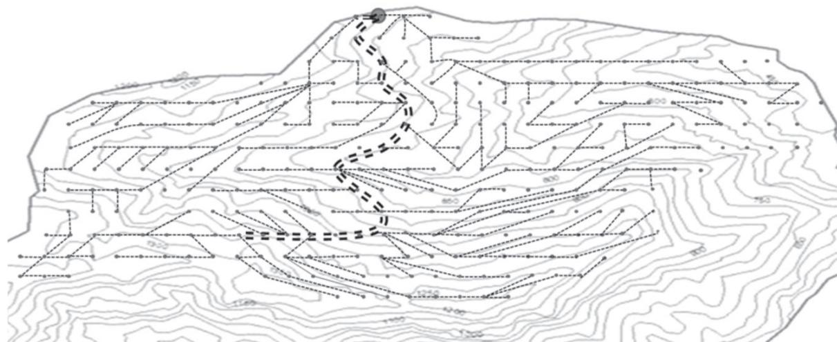
**Fig. 7** Solution showing the road and related access spurs ( $R_{fact} = 1.0$ )
