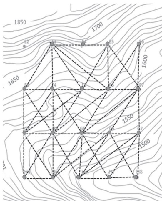
**Fig. 5** Access spur feasibility; there may not be 20 links for each node because of steep terrain, swamp areas, or no volume at the systematically placed harvest node
