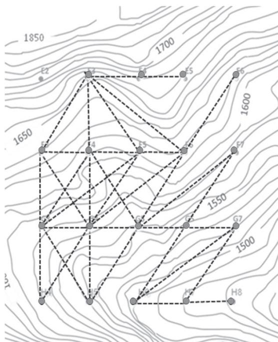
**Fig. 4** Typical road feasibility; due to slope, swampy areas, or no volume to be extracted, there are typically less than 20 links for each node
