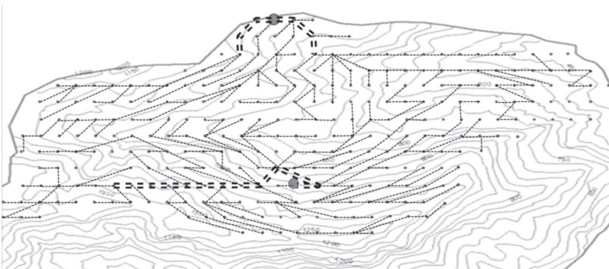
**Fig. 9** Solution showing the road and related access spurs ( $R_{fact} = 1.00$ , 2 Exit Points)
