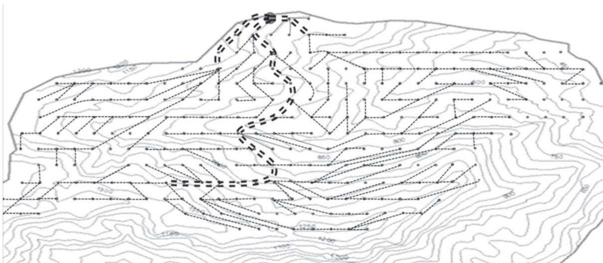
**Fig. 8** Solution showing the road and related access spurs ( $R_{fact} = 0.70$ )
