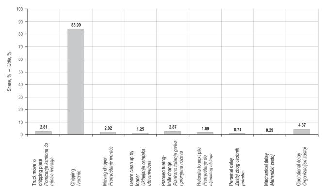
Fig. 4 Time breakdown (% of working time) for chipper
