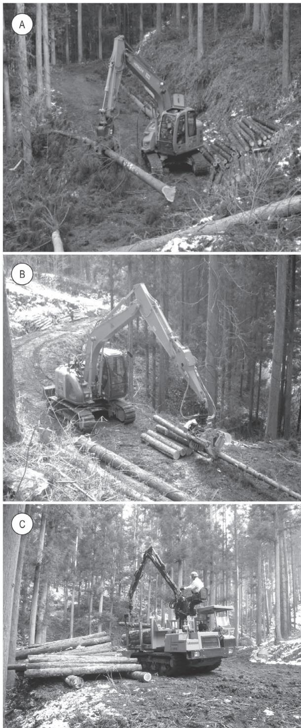
**Fig. 2** Operational system with grapple-loader bunching (A), processor processing (B), and forwarder forwarding (C)
