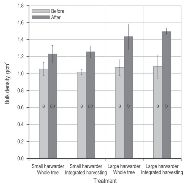
**Fig. 3** Average soil bulk density before and after machine activity for the four analysed treatments ( $n=3$  per column, the error bars represent the standard deviations). Columns that do not share any letter are significantly different ( $p \leq 0.05$ ) according to Tukey's HSD tests of means
