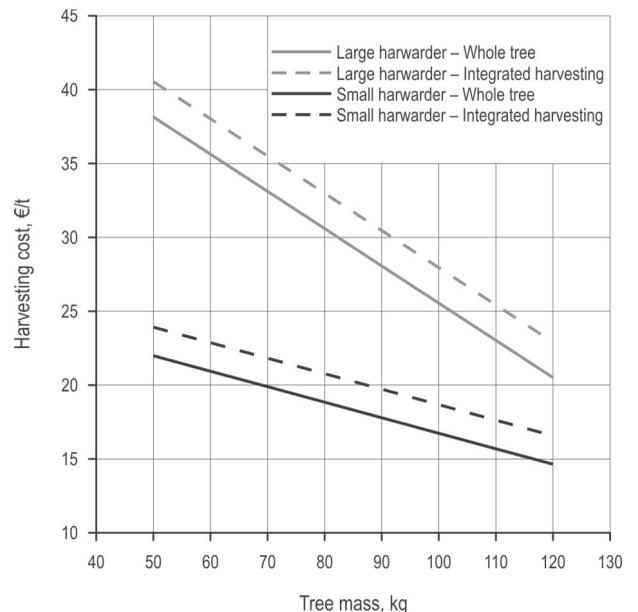
**Fig. 1** Harvesting cost as function of tree mass for the four different treatments (calculated using Eqs. 2 – 3 with the average removal fresh mass set to 45 t/ha)
