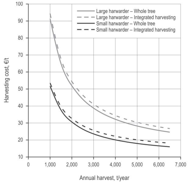
Fig. 4 Harvesting cost as a function of annual harvested biomass. (Calculated with the average removal fresh mass set to 45 t/ha and average removal tree fresh mass set to 82 kg)
