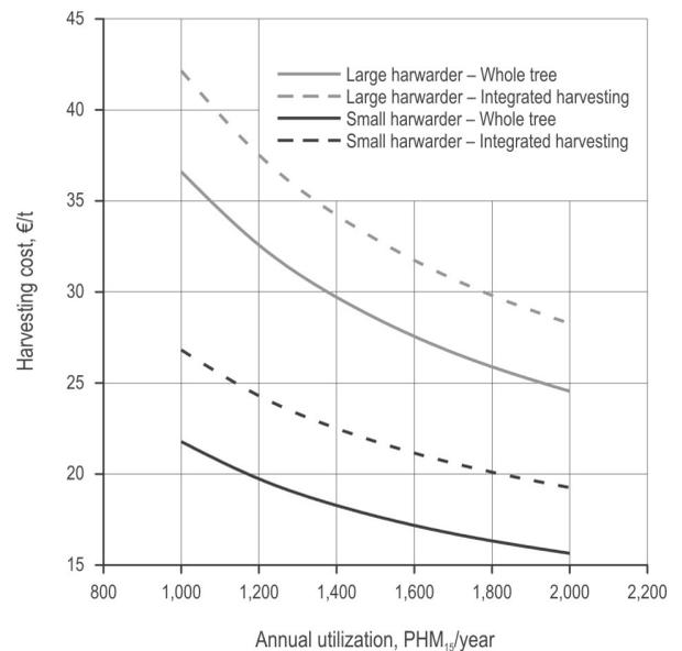
Fig. 5 Harvesting cost as a function of annual usage of harwarders for four treatments. (Calculated with the average removal fresh mass set to 45 t/ha and average removal tree fresh mass set to 82 kg)
