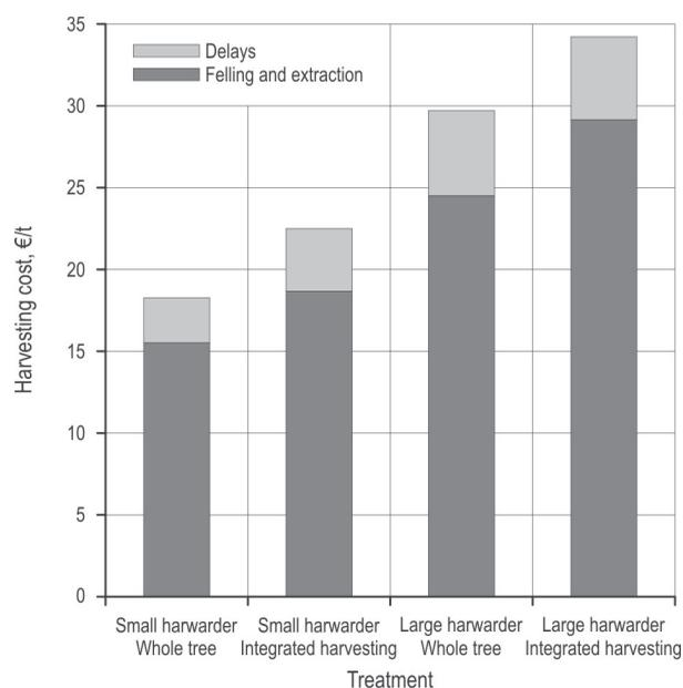
**Fig. 2** Average harvesting cost by treatment and activity in the field study. (Calculated with the average removal fresh mass set to 45 t/ha and average removal tree fresh mass set to 82 kg)
