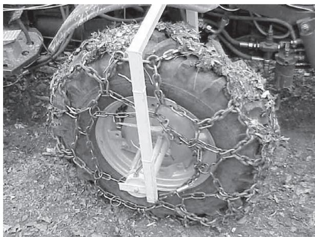
**Fig. 7** Chains on a tractor drive wheel
