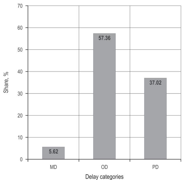
**Fig. 6** Delay time distribution by categories (*MD*: Mechanical delays, *OD*: Operational delays, *PD*: Personal delays)
