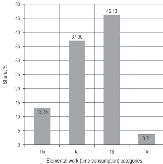
**Fig. 4** Structure of elemental time consumptions (%) within a delay-free on-road skidding work cycle (*Tla*: Time consumption for load attachment, *Tet*: Time consumption for empty travel, *Tlt*: Time consumption for loaded travel, *Tld*: Time consumption for load detachment)
