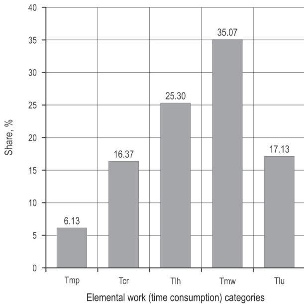
**Fig. 3** Structure of elemental time consumptions (%) within a delay-free winching work cycle (*Tmp*: Time consumption for manoeuvring and parking, *Tcr*: Time consumption for cable releasing, *Tlh*: Time consumption for log hooking, *Tmw*: Time consumption for mechanical winching, *Tlu*: Time consumption for log unhooking)
