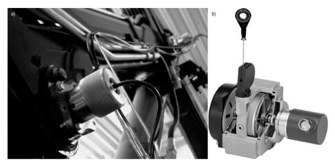
Fig. 2 Joint angle sensors with quadrature optical encoders: a) Encoder mounted on a joint; b) Rotary encoder with wire box for measuring linear motion (source: http://www.tfe.umu.se)
