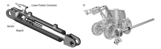
Fig. 1 Position sensing for hydraulic cylinders: a) A linear position sensor; b) Linear position sensor on a machine (source: www.texashydraulics.com)
