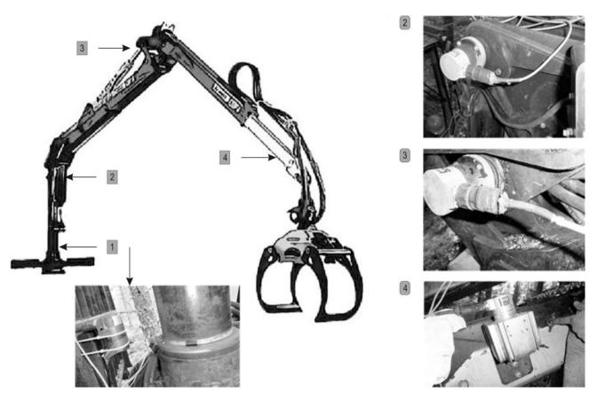
**Fig. 6** Forwarder crane with sensors attached at the joint level for measuring angular motion. This experimental platform has been operating for more than a decade. During this time the sensors have never been changed. Based on this demonstration of the sensing device's reliability and robustness, a commercial version of this solution has been developed (Cranab 2013b)
