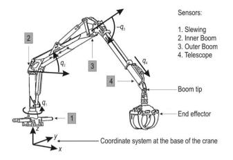
Fig. 7 Forwarder crane coordinate system and generalized joint coordinates
