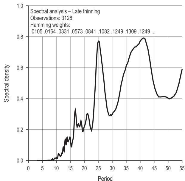
**Fig. 3** Fragment of a periodgram of harvester work in late thinning. The highest peak of the periodgram indicates the strongest work cycles
