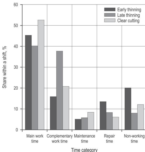
Fig. 1 Time structure of a harvester working shift
