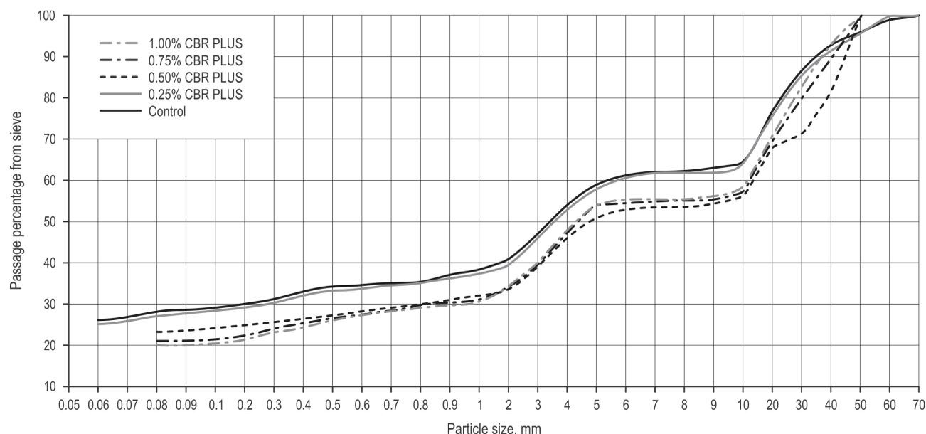
**Fig. 4** Curve of weight distribution of particle size for materials treated by different percentages of CBR PLUS
