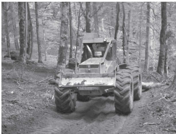
Fig. 2 Rubber-tired skidder (Timberjack 450C) used in logging operations in a mountain forest of Iran
