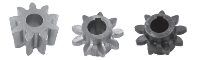
Fig. 2 Sintered gear after compaction and sintering (left), after machining (middle) and after heat treatment (right)
