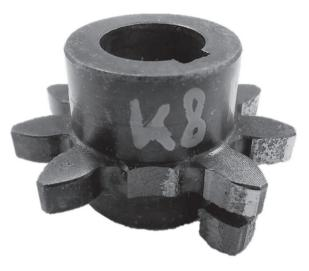
**Fig. 8** Typical damage after test – test gear K08
