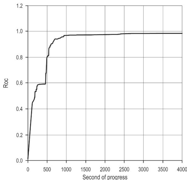
Fig. 3 Pothole ROC Curve in ANN model
