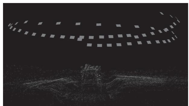
**Fig. 3** Sparse point cloud generated with Agisoft PhotoScan
