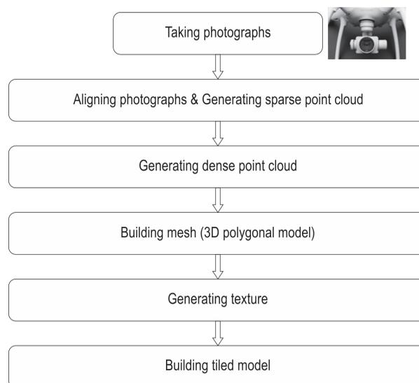
**Fig. 2** Agisoft PhotoScan's project workflow for image processing and 3D reconstruction
