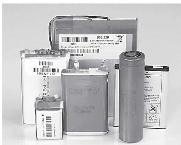
Fig. 3 Different shapes of Li-ion battery
