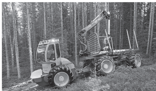
Fig. 10 Elforest – hybrid forwarder ( http://elforest.se )
