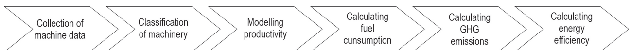
Fig. 1 Procedure for producing fuel consumption, GHG emission, and energy-efficiency figures for the forest machine fleet of the study
