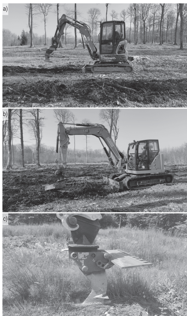
Fig. 1 (a) Small excavator; (b) Large excavator operating during the wet period; and (c) Close view of the tool mounted on the large excavator
