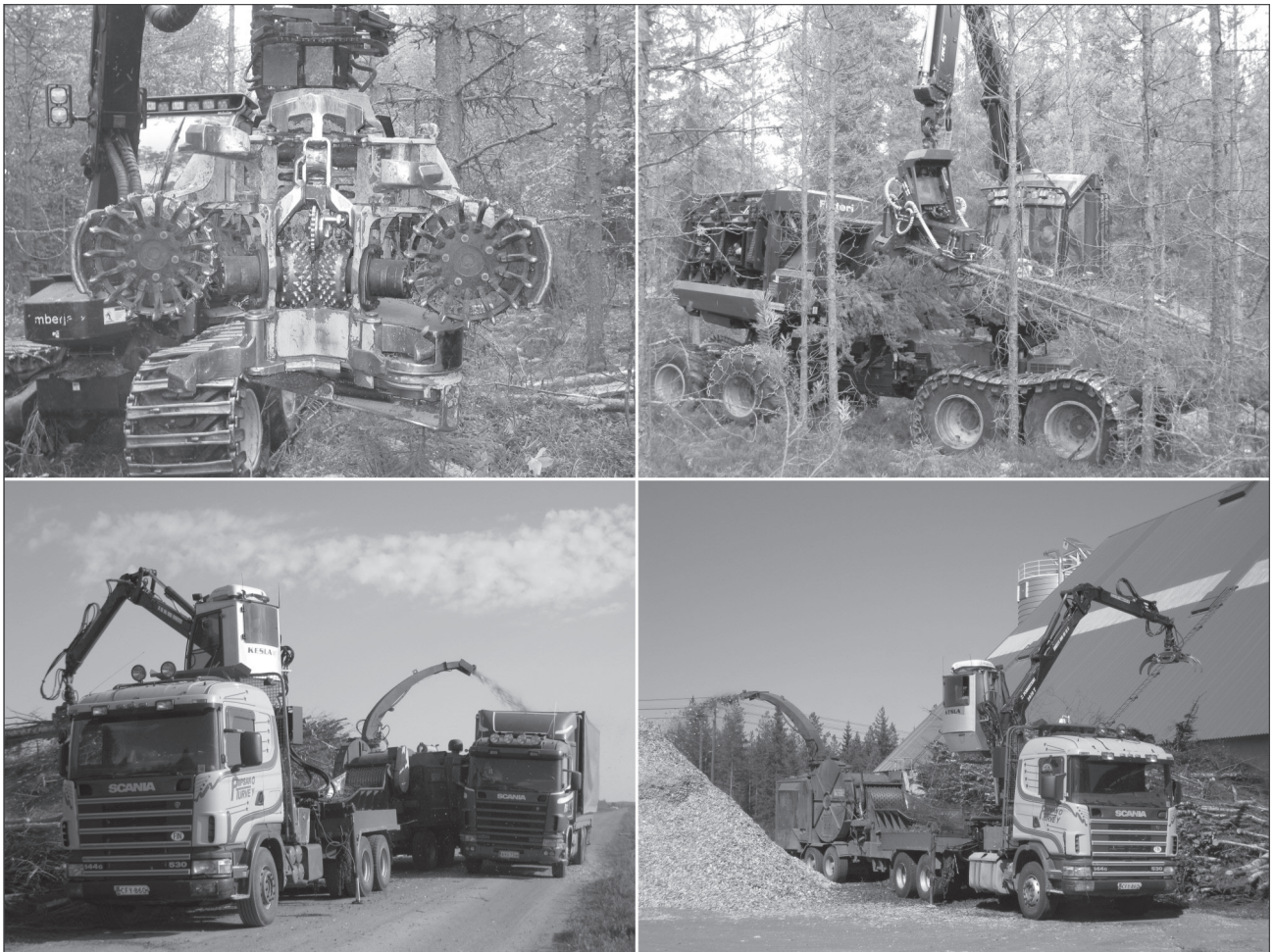
Fig. 1 A conventional harvester head equipped with multi-tree-handling accessories (up) and Fixteri II bundle harvester. Chipping of energy wood at a roadside landing or at a terminal using a trailer-mounted drum chipper (down)
