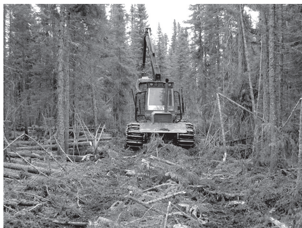
Fig. 1 Forwarder operated over a brush covered machine operating trail Slika 1. Forvarder na traktorskoj vlaci pokrivenoj zastorom granjevine
