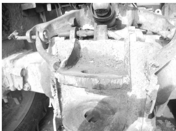
Fig. 2 Damaged drawbar bracket of Massey Ferguson 375 tractor
