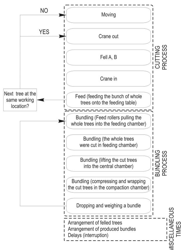
**Fig. 2** Flow chart of work processes for the studied bundle-harvester (cf. Nuutinen et al. 2011, Nuutinen and Björheden 2015). Fell A, B indicate that the work can include accumulation of several trees
