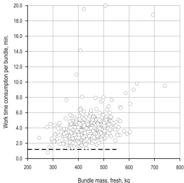
**Fig. 6** Time consumption to produce a bundle as a function of the bundles mass. The dotted line indicates the maximum capacity of 1.2 min/bundle, reached for bundles with masses between 400 and 500 kg in the study. Values of time consumption lower than ca. 7 min are considered as PM<sub>0</sub> time, i.e. work with no delays
