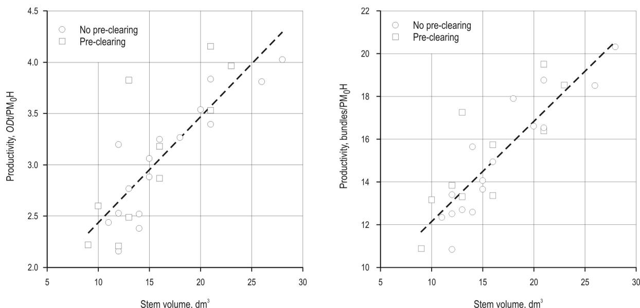
**Fig. 4** Productivity (to left, *OD* t/PM<sub>0</sub>H and to right, bundles/PM<sub>0</sub>H) of the bundle-harvester system as a function of average size of harvested tree
