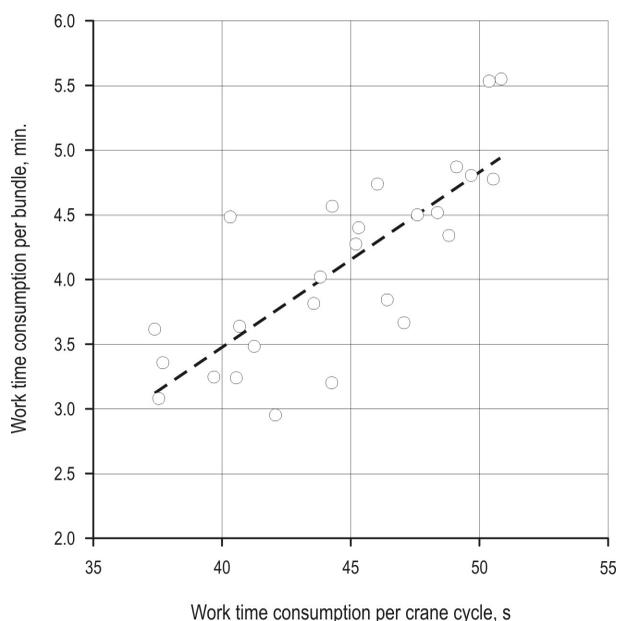
**Fig. 3** Time consumption (PM<sub>0</sub>) of the bundle-harvester to produce a bundle as a function of time consumption per crane cycle work. Calculations are based on average values for 26 time study plots
