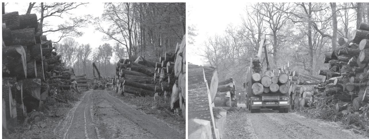
**Fig. 10** Typical forwarder roadside landing
