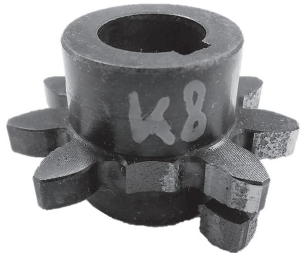
Fig. 8 Typical damage after test – test gear K08
