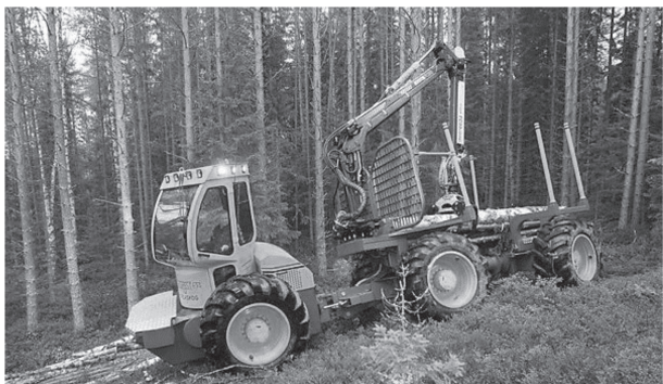
Fig. 10 Elforest – hybrid forwarder ( http://elforest.se )
