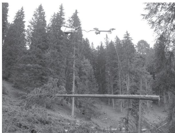
Fig. 1 Example of a double-hitch carriage. While stems and/or logs can be attached separately to each dropline, connecting to both ends of a tree allows the tree to be extracted horizontally
