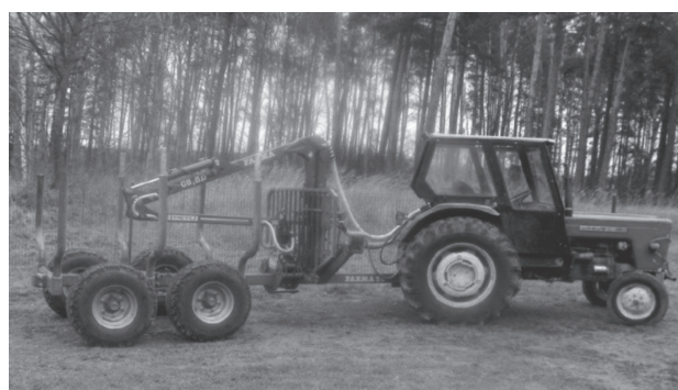
Fig. 1 Forwarding unit: Ursus C-360 tractor with Farma T6 trailer
