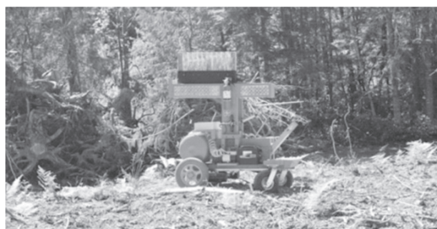
Fig. 6 Model of a remote-controlled forest planting automatic device
