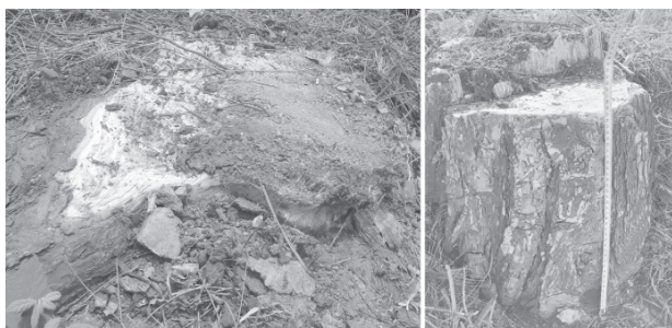
Fig. 2 Sample stumps cut with feller-buncher (left) and with chainsaw (right)
