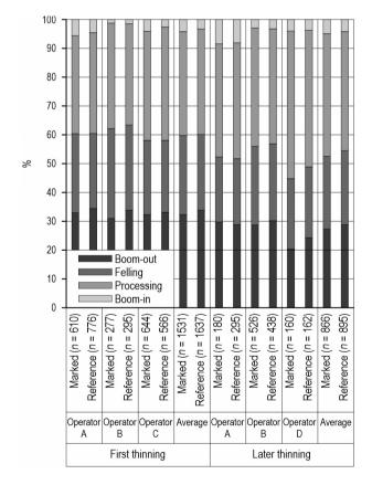
**Fig. 4** Distributions of work elements of boom-out, felling, processing (delimbing and cross-cutting) and boom-in of total effective time by treatment, operator and thinning type
