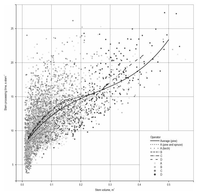
Fig. 6 Curve modelled for stem processing time (i.e. felling, delimbing, cross-cutting and boom-in) as a function of stem volume removed (Tables 5 and 6)
