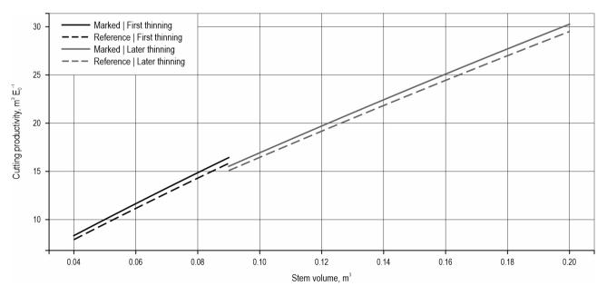
**Fig. 7** Cutting productivity in marked and reference first and later-thinning stands as a function of stem volume removed. Removal density used was 800 stems ha<sup>-1</sup> in first thinnings and 300 stems ha<sup>-1</sup> in later thinnings
