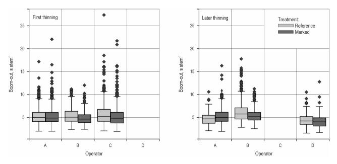
Fig. 5 Boxplot figures of time consumption of boom-out in first and later thinnings by operator and treatment, showcasing distributional characteristics (i.e. minimum, maximum, and first and third quartiles) of each operator and possible outliers
