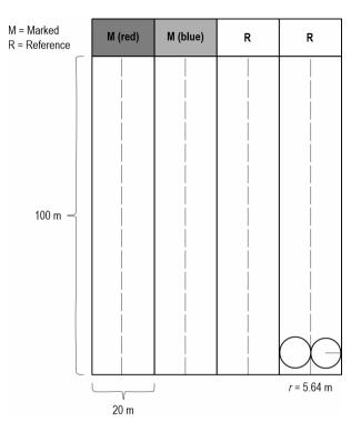
**Fig. 2** Layout of time-study plots. Each plot was 20 m wide, with varying length (100 m in this example). Thinning intensity of reference stands was measured from circle plots (r = 5.64 m)
