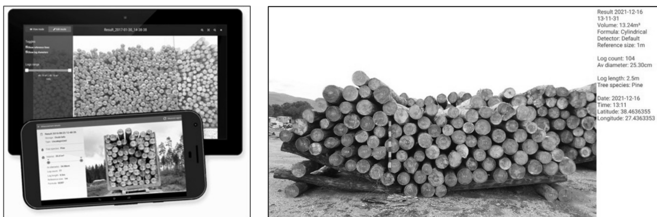
Fig. 3 View of Timbeter mobile app and view of the app during measurement (Timbeter 2021)
