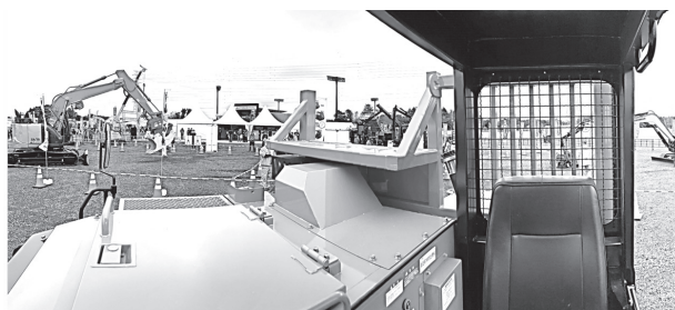
Fig. 1 Forwarder large blind spots from the operator's working position. These blind spots, created by the vehicle itself, can lead to delayed hazard avoidance, resulting in an increased risk of accidents
