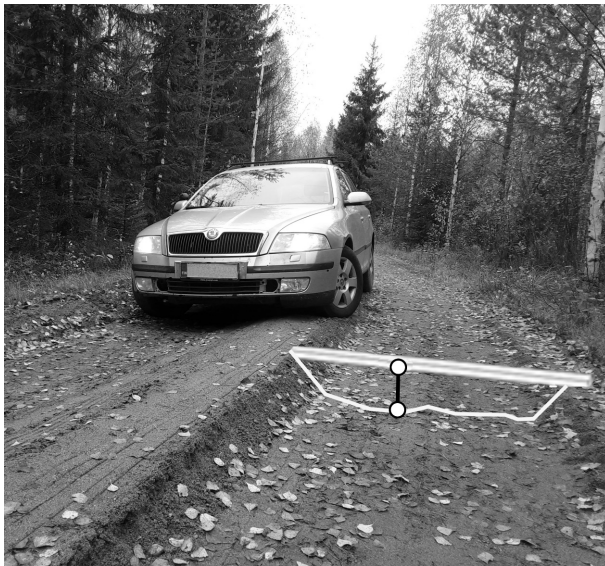
Fig. 3 Schematic view of the applied collection method. White bar represents a straight pole, white line the road surface profile. Maximum distance between road profile and pole is indicated by black line
