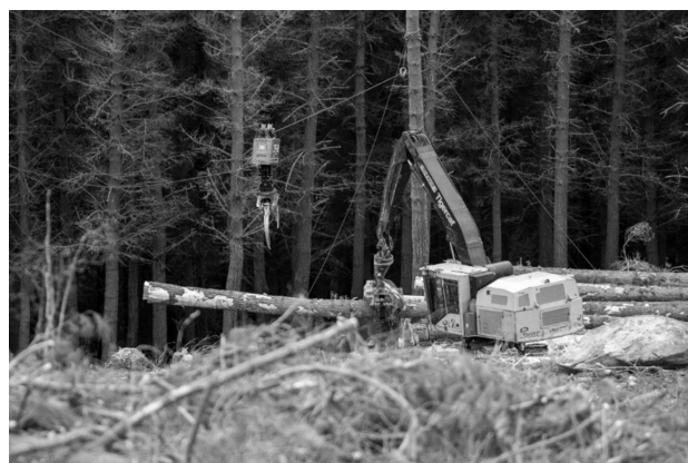
Fig. 2 Tigercat LS855E feeding a stem to Falcon 1750 at Site # 2 (Geraldine)
