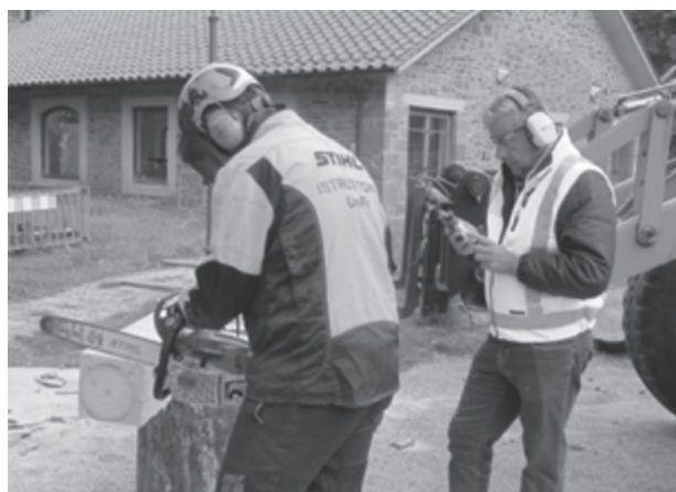
Fig. 5 Vibration measurements during cross-cutting
